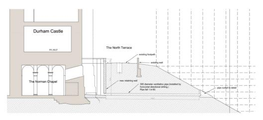
Fig 3. Side profile showing proposed lightwell and ventilation pipe
