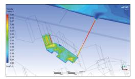
Fig 4. CFD (Computational Fluid Dynamics) simulation testing the air flow and how it will be drawn in to dry out the north wall of the Norman Chapel.
