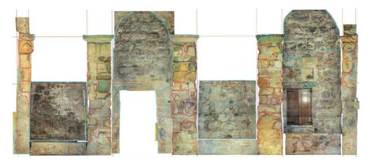
Fig 2. The condition of the stones recording by Hirst Conservation.
